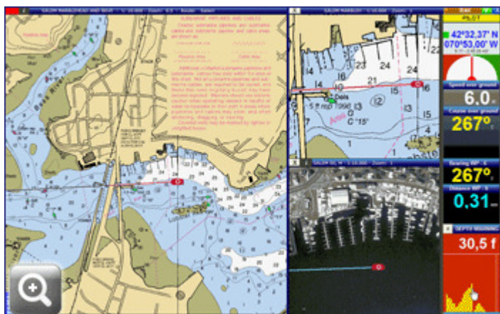
TIKI can simultaneously display one, two, or three chart windows. In this example a chart overview (left) and zoom (top right) are complemented by a satellite photo (bottom right).
